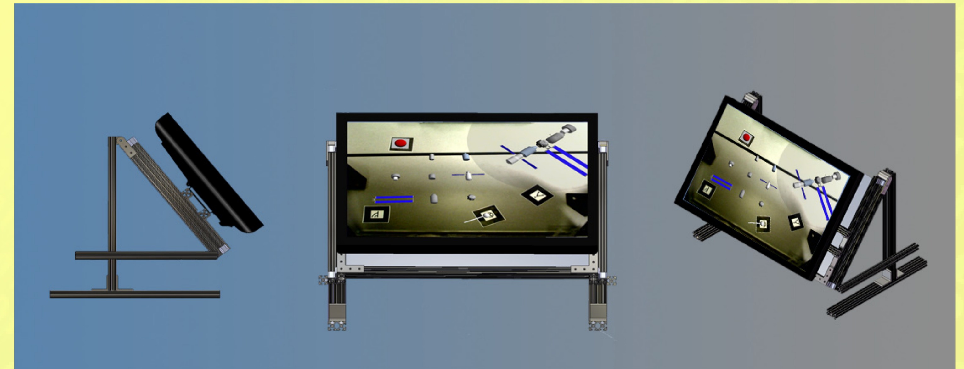
Three Dimensional CAD drawings of the Magic Table. The user manipulates the wand to move pieces to the build site. The parts library, wand, reset button, and build site are all displayed.
