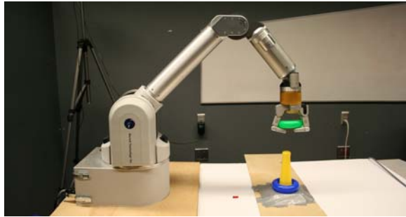
Figure 5: View of the remote arm under the control of the primary arm during the ring stacking task.
