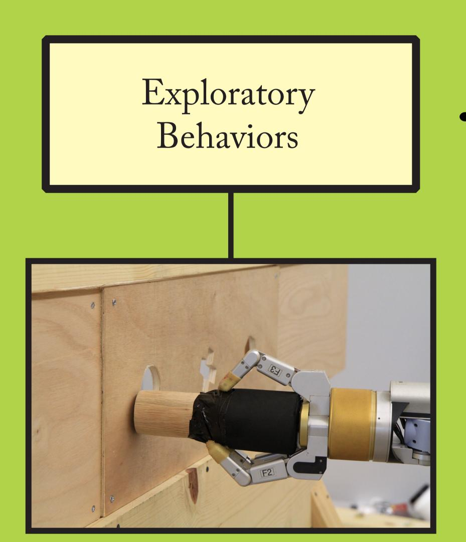
The robot pushes the board with a block until it is stuck. The robot then explores the region around the hole using pushing behaviors. The robot makes 5 attempts to fit the block. If it achieves a fit, 5 additional pushing behaviors are performed to explore the 'fit' state. 20 of these trials are performed for every block and hole combination.
