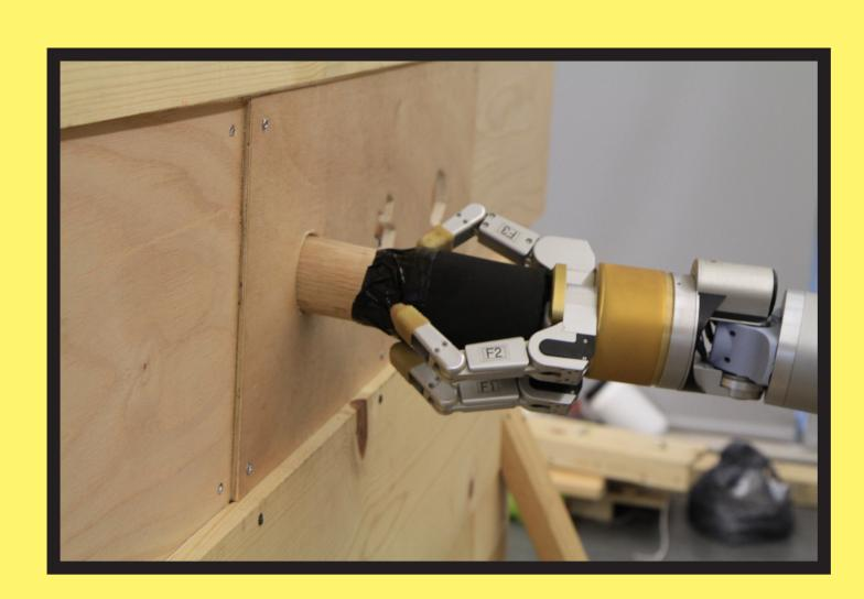
The robot fit the block with 15%-50% success, depending on the shape.
