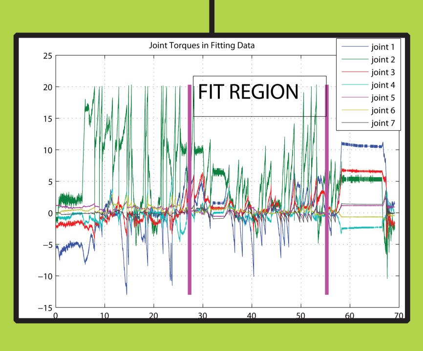
During exploration, robot records joint positions, joint torques, audio, and video. This data is time-stamped. The human experimenter detects when the robot has fit the block, signals the robot to perform additional pushing behaviors, and marks the data accordingly.
