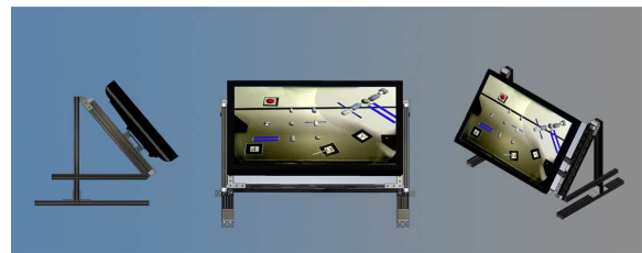
Figure 8: The left, front, and isometric SolidWorks views of the final design. The side bars are clamped to the user's desired height and can be adjusted via the top pivots.
