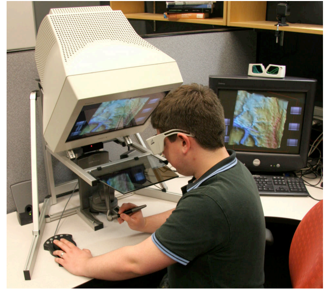
Figure 4. Using a collocated setup where active stereo graphics are displayed onto a mirror, beneath which the phantom is operated
