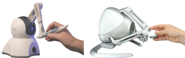
Figure 3. Low-end point force feedback devices: Phantom Omni(left ) and Novint's Falcon (right)
