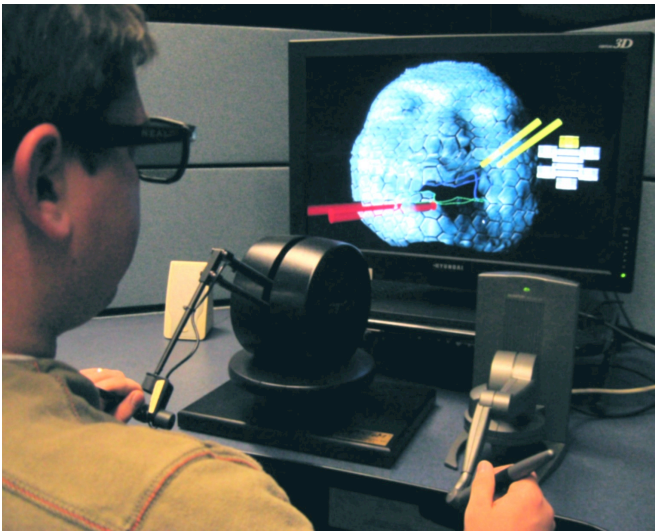
Fig. 1: The M4 system is used to directly manipulate a textured, irregular triangle mesh with two haptic devices.
