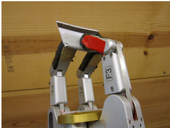
Fig. 4. Tape used to enhance the robot's grasp on the card.
