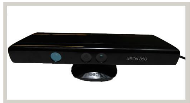
Figure 2: The Microsoft® Kinect™ is a COTS device that operates via touch-free navigation.
