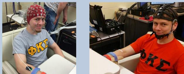
Figure 1. Traditional wired and dry wireless EEG systems.
