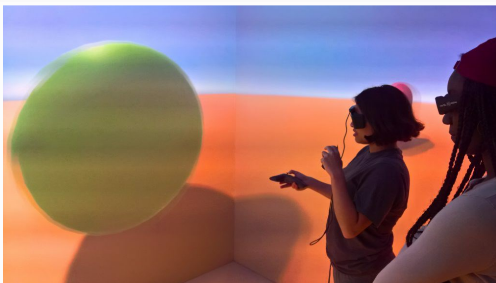
Inside the C6. The Cave is calibrated for the wearer of the main 3d glasses, in this case Devi.
